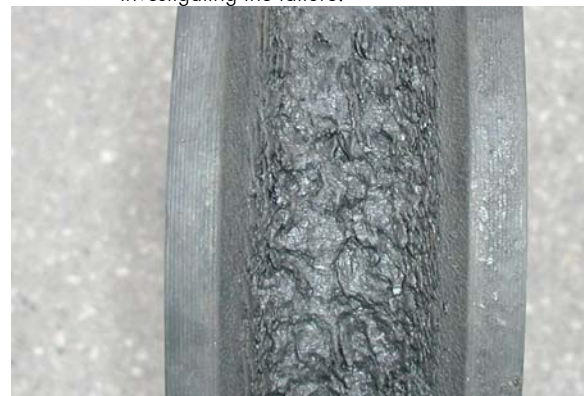
Typical damage of improper use of grease
