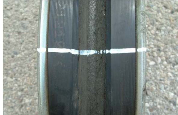
Method to check gliding of the sheave liner
