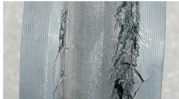
Thermal corrosion of sheave liners
